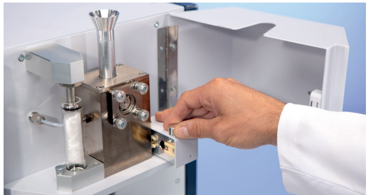
Electrode furnace with SampleCare™ and FusionControl for real-time sample temperature detection, Bruker only.
